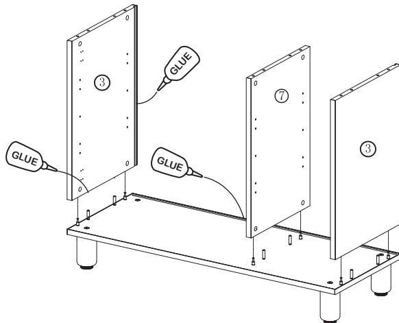
EN add glue to wooden dowel holes and slot of ⑦ .
