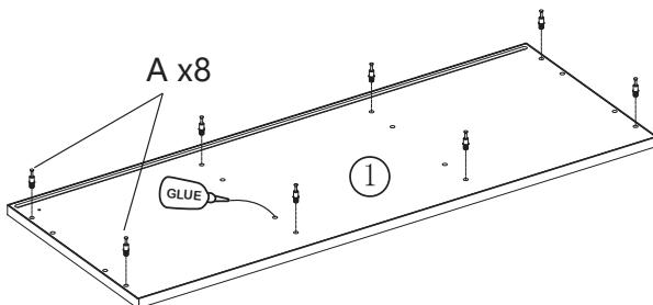
EN add glue to wooden dowel holes and slot of ①.
