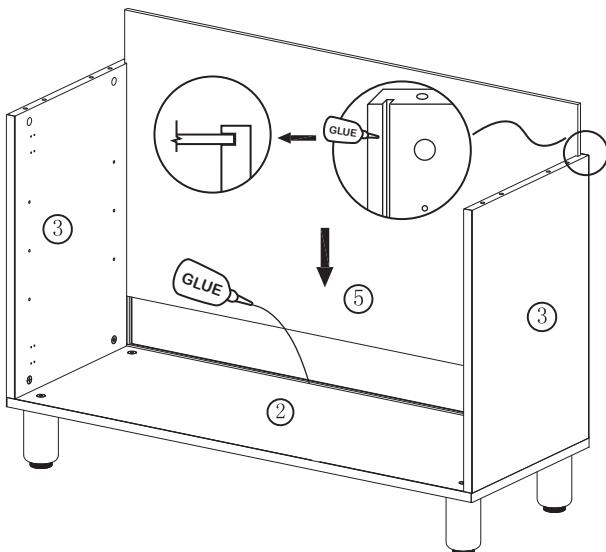
EN add glue to wooden dowel holes and slot of ② and ③.
