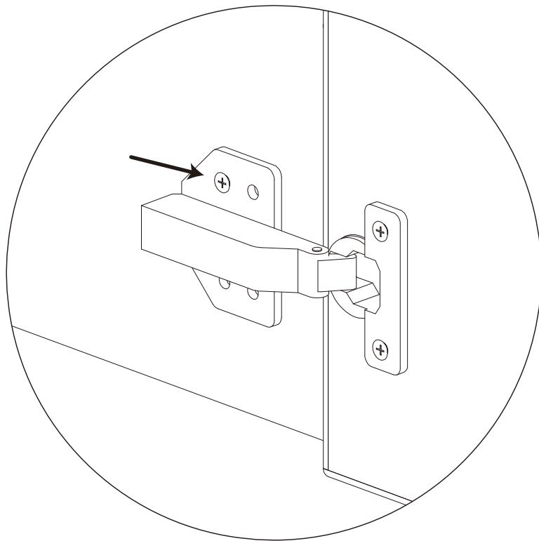
EN you can adjust the doors by loosing the screw pointed.
